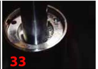
29. Use your fingers to start pushing in the blue seal, after about half way you will need the assistance of your seal pick and carefully press in the seal, air and oil will be trapped under the seal so the very last part of the seal needs to have the seal pick gently pushed in between the side of the seal and the housing to release the last bit of excess oil and air. ( Image 34 )
