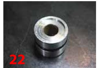
22. Once you have done the rod guide push on the neck bush, blue seal, rod guide and the piston assembly in reverse of the way they come of the shaft. Apply Lock tight to the thread and tighten the nut to 30 NM for the 10mm nut or if your shock uses a 12mm nut tighten to 50 NM. With all the O-Rings and seals replaced with new items it is now time to replace the High Pressure line.
