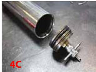
5. Using both hands depress the alloy retainer down enough to remove the circlip with a seal pic. ( image 4)
